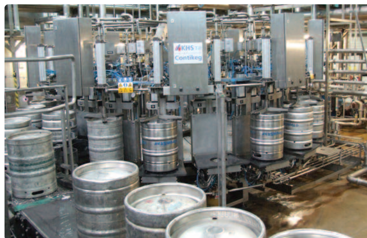
Figure 11 left: A rotary keg filling line – a popular choice for keg lines of over 500 kegs/hr.
