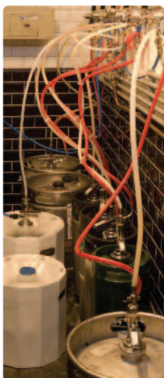
Figure 8: A PET KeyKeg on dispense in a beer cellar. Photo: Lightweight Containers
