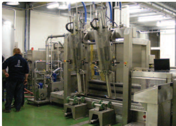
double head capable of up to 60 and 120 casks per hour (Figure 13).
