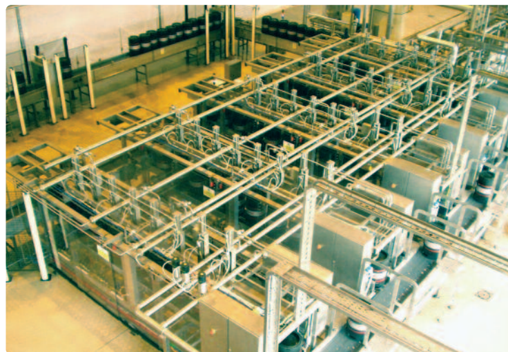
Figure 12: A 5-lane B&R keg machine installed at the new Grolsch Brewery in 2003. The 550 kegs/hr line is very flexible and easy to work on when in production.
