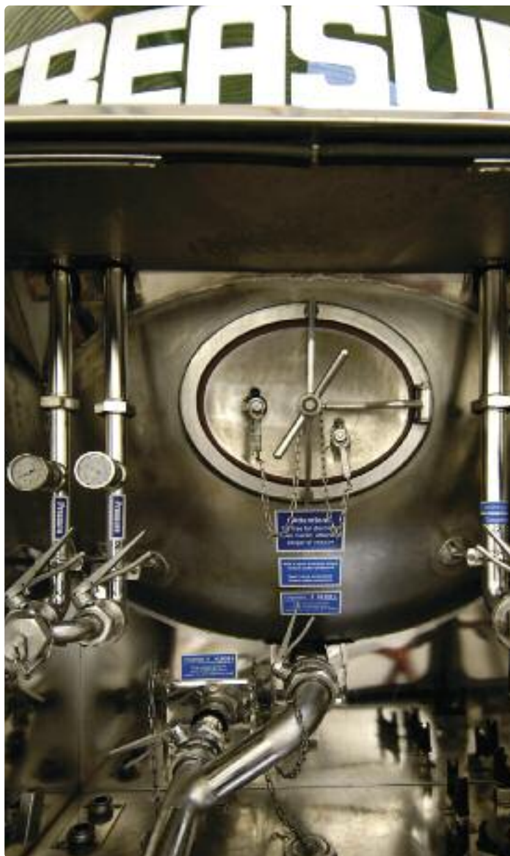
Fig 6: General view of the back of a beer tanker, showing beer, CIP and top pressure connections.
