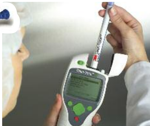
Fig 7 left: Clean-Trace bioluminescence probe for sampling swabs and rinse liquors. Photo: 3M Ltd
