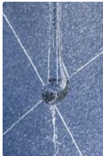
LEFT: Fig 4: Spray pattern from a high pressure low volume rotary jet.
