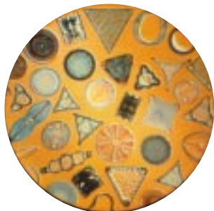
The diverse nature of kieselguhr as seen under a microscope.
