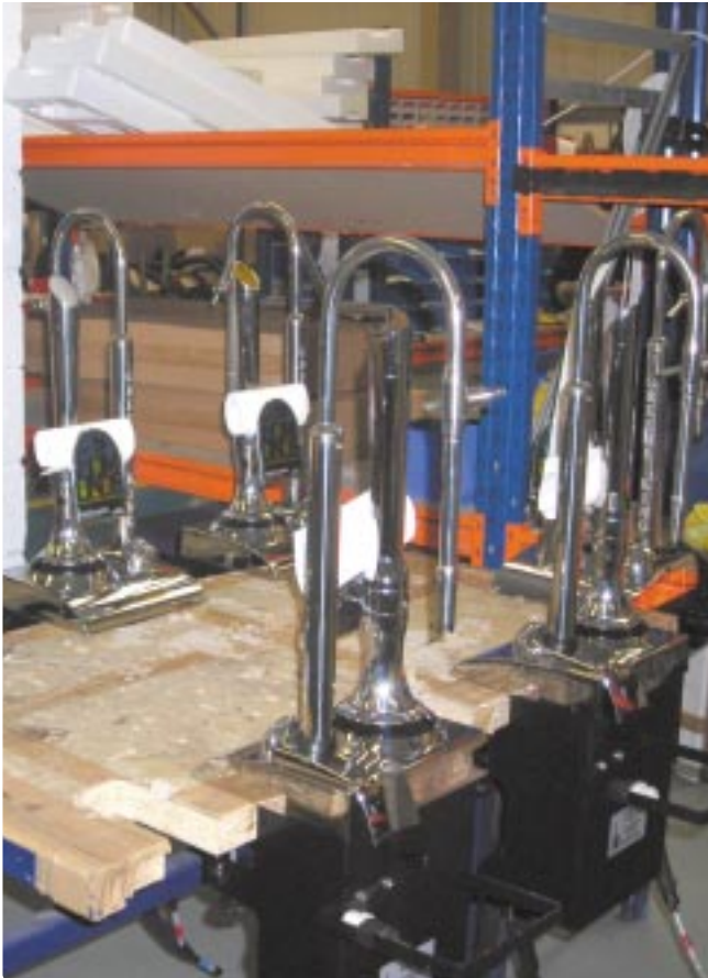
New quarter-pint Musketeer beer engines for Greene King's new St Edmunds cask ale in final testing at DDg.
