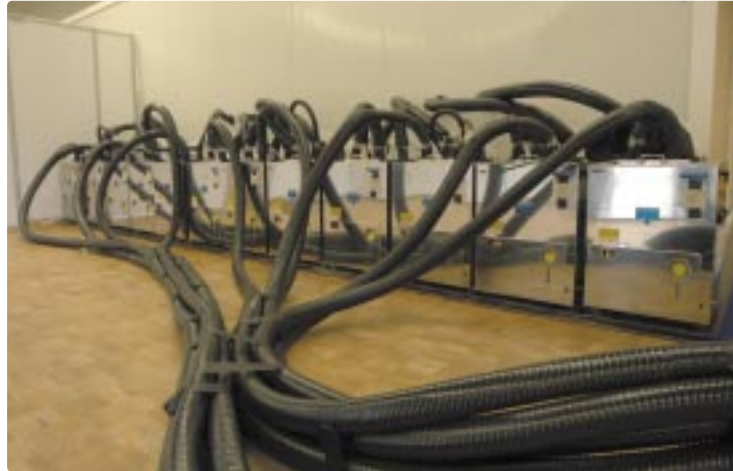
The pythons used at the Brewing Industry International Awards at Drinktec last year to cool beer to over 100 taps.
